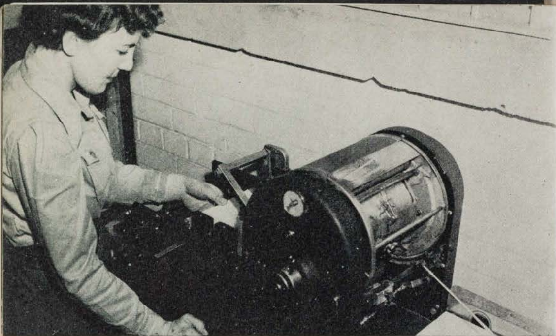
This machine prints the letters and orders from stencils prepared by WAAC typists. A skilled operator is needed to run the high-speed mimeograph machine. This WAAC mimeograph operator is a specialist who has replaced the soldier who formerly did this work.
