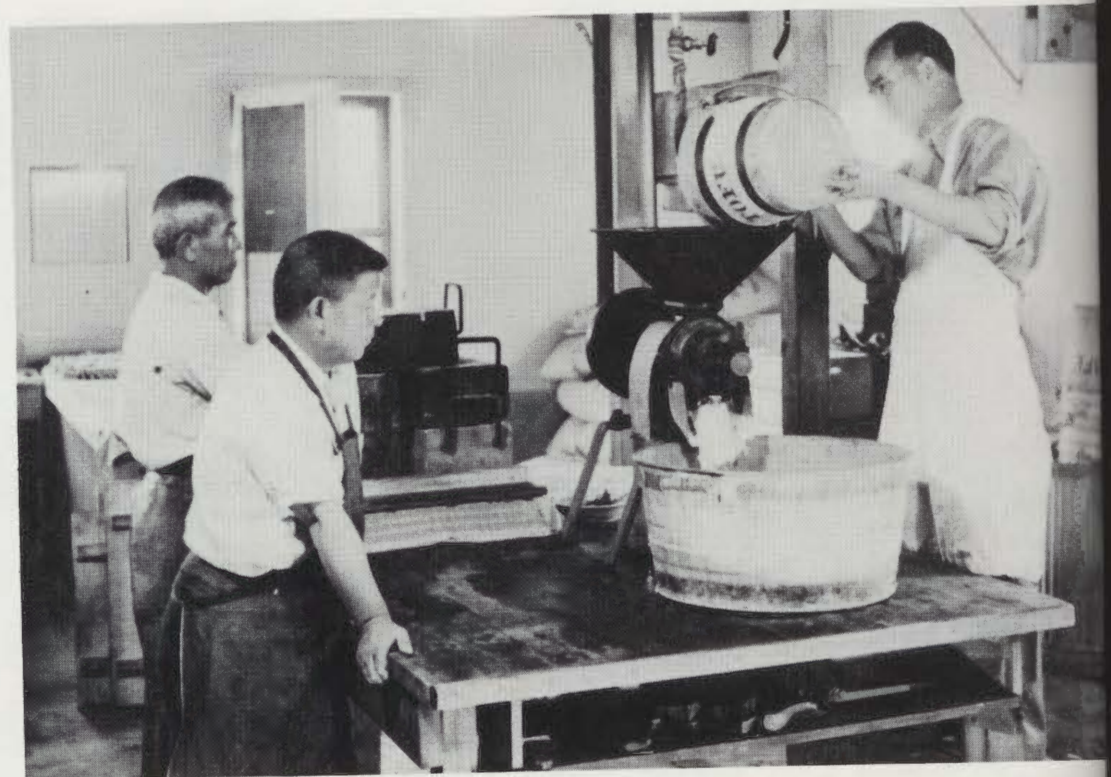
Tofu factory: funyu press - extract funyu from cooked and ground soy beans
