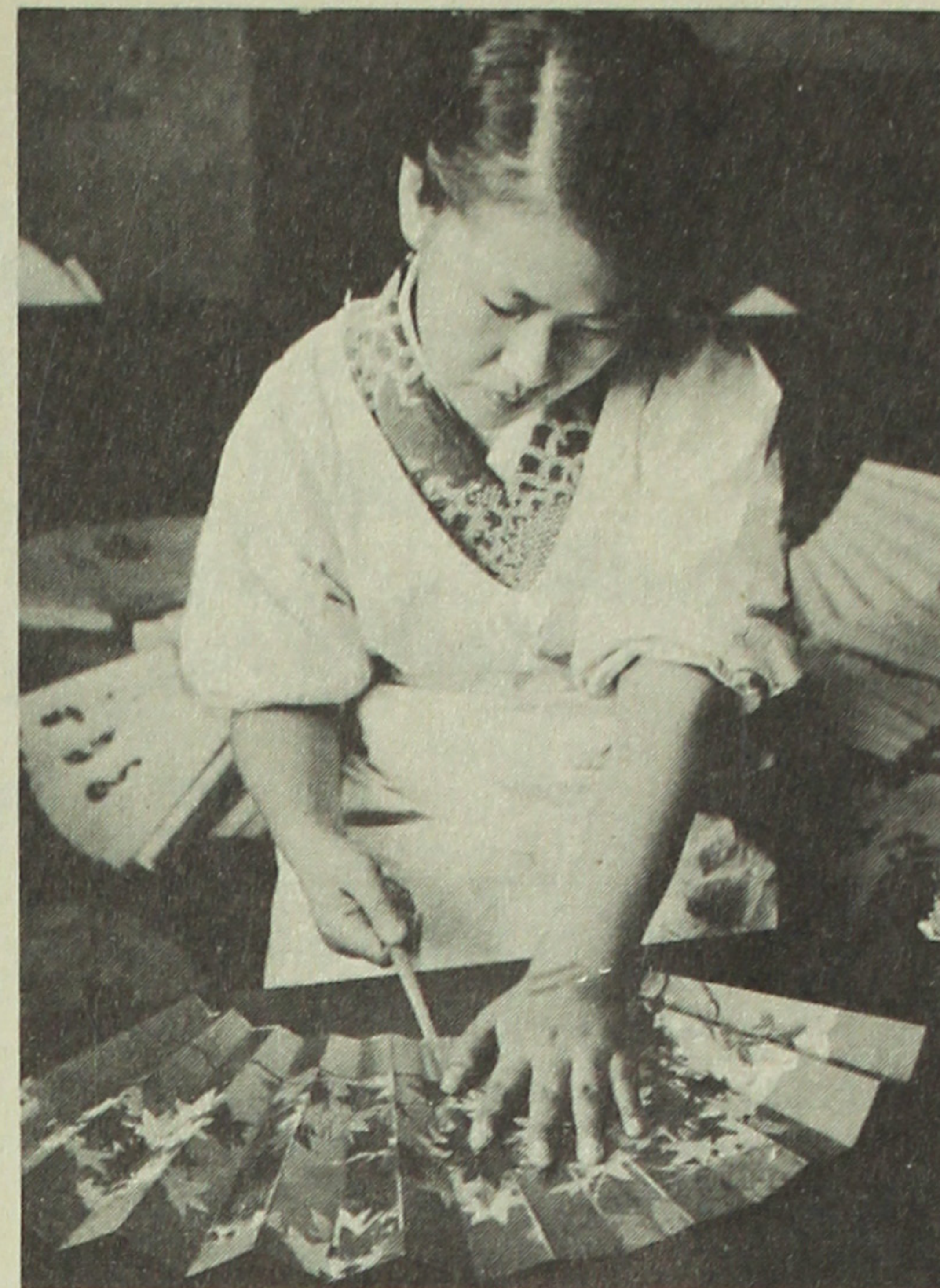
SLOTS are made in fan's paper covering. When ribs are fitted into slots, fan is completed.
