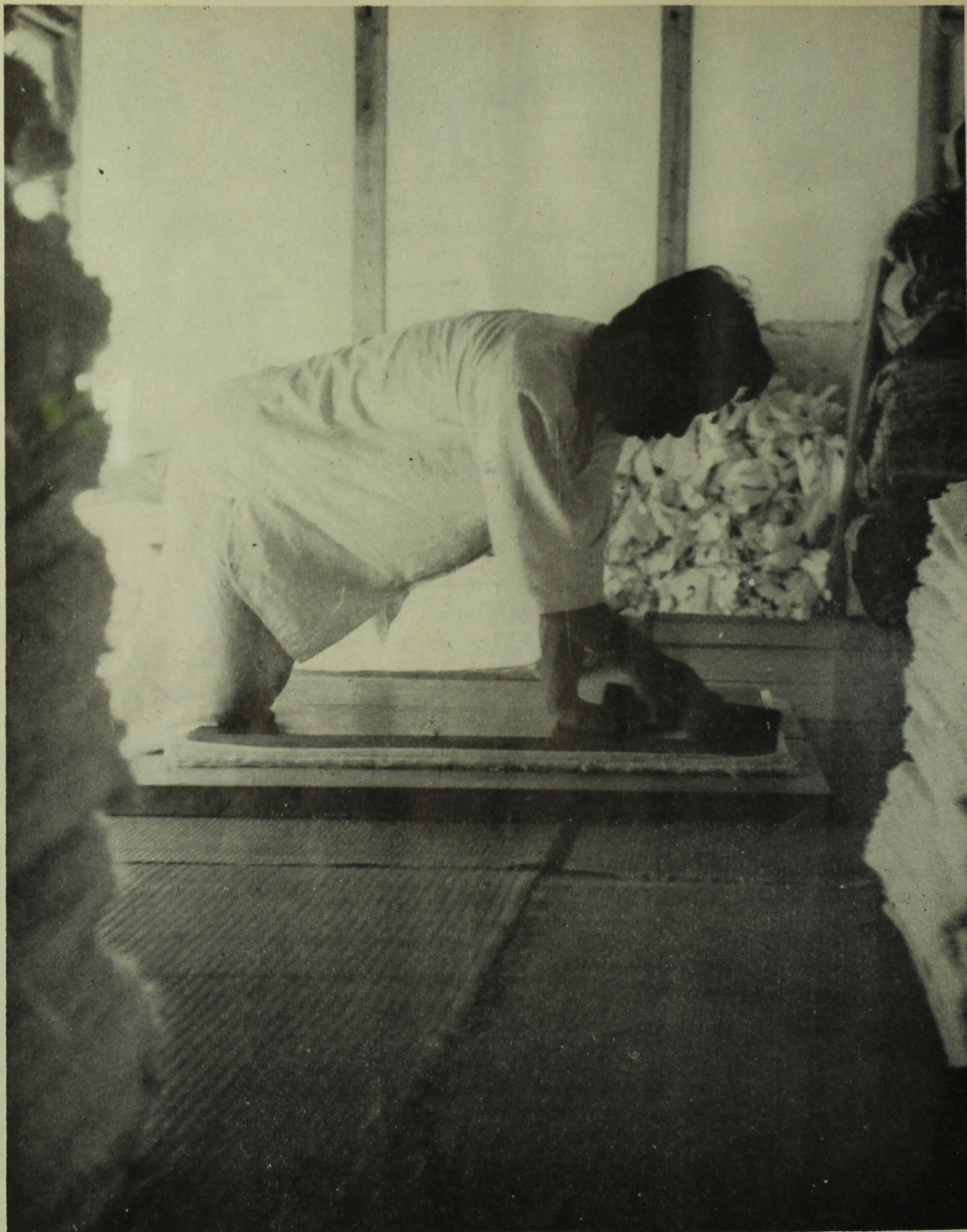
STACKS OF FINISHED PAPER are trimmed by hand with a sharp knife, packaged with straw rope, shipped to market.
