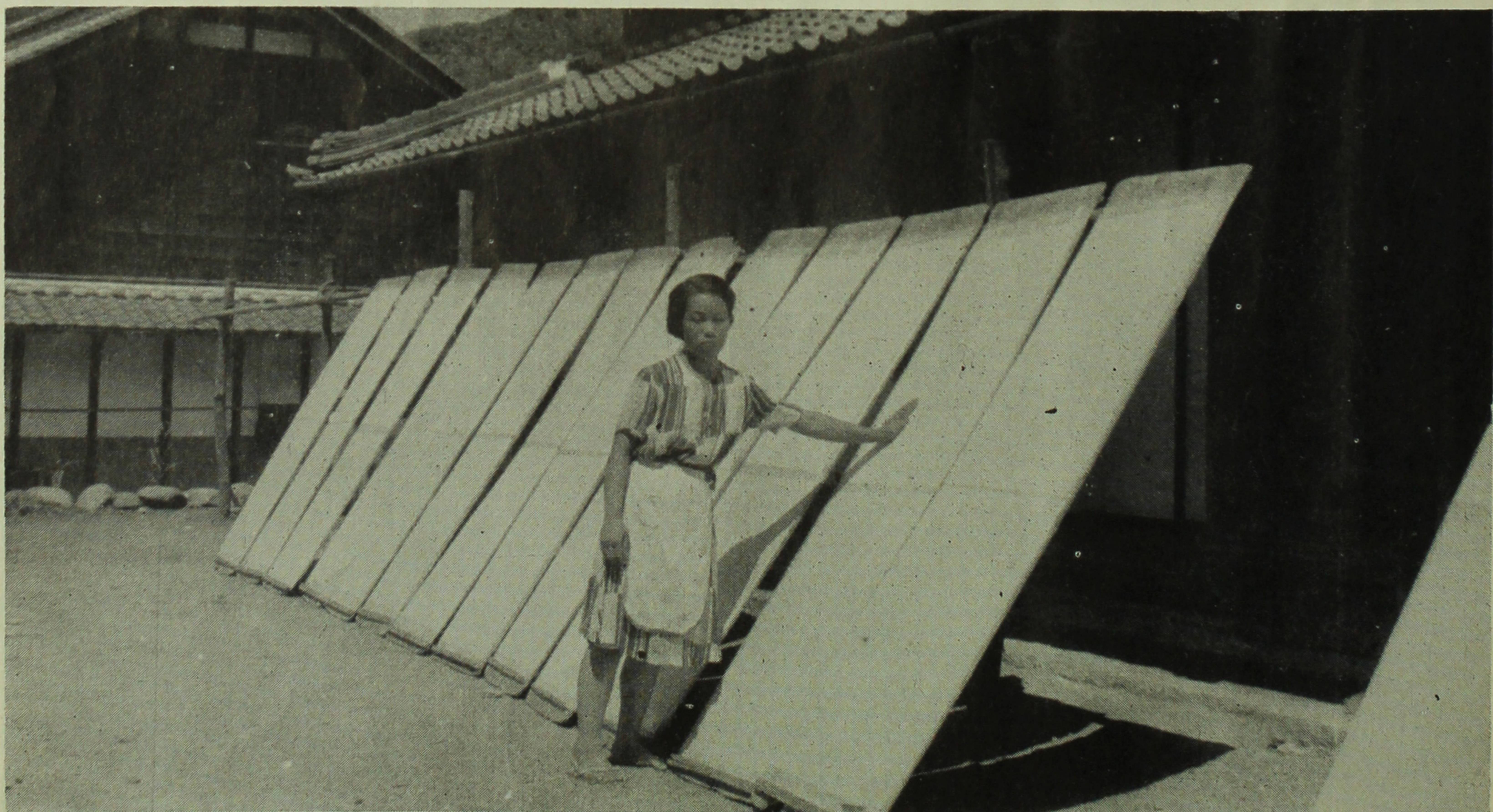
SMOOTH SURFACED DRYING BOARDS dry paper in the sun; side near board is smooth; brushed side is rough.
