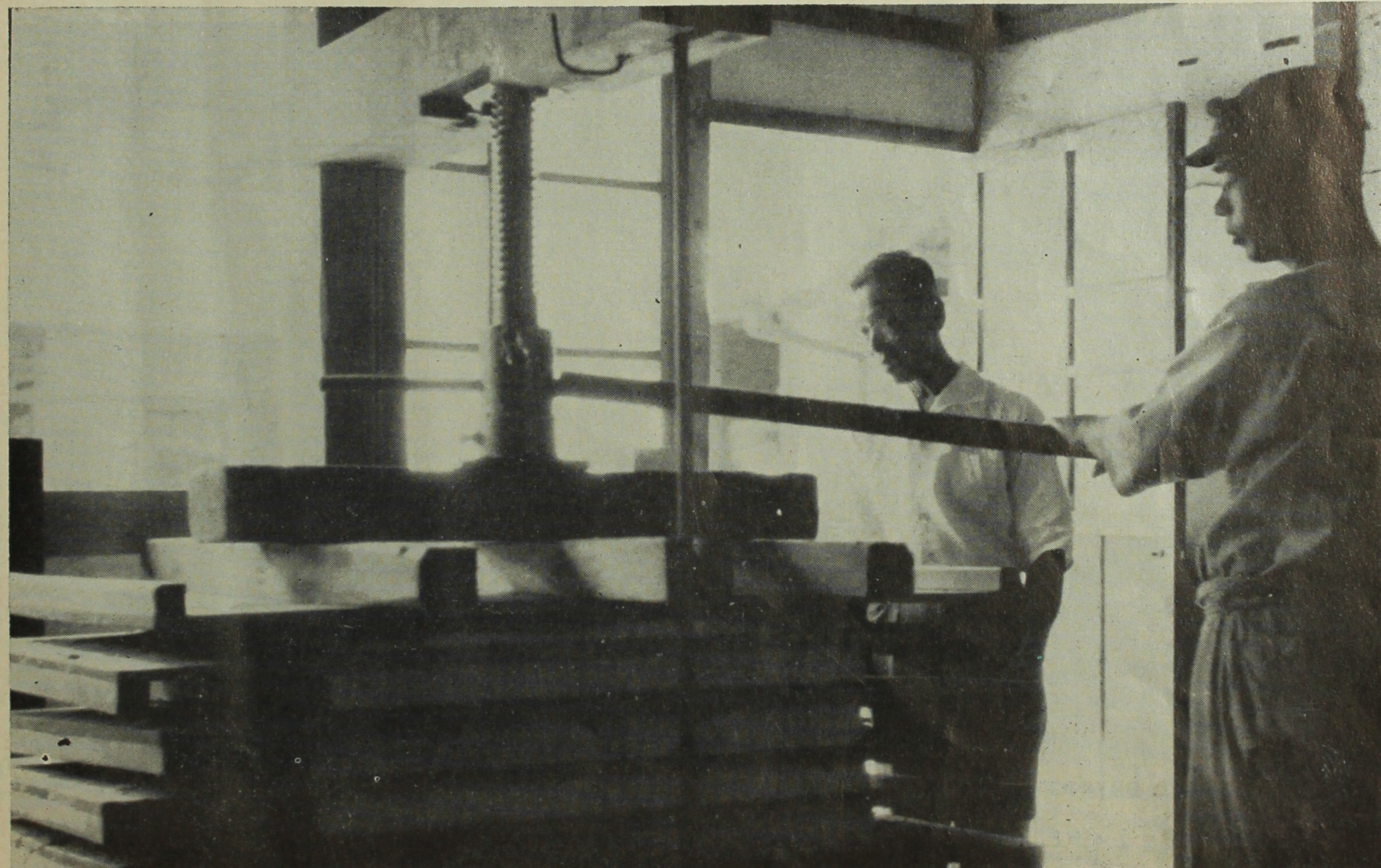
HAND OPERATED PRESS or a stone press is used to squeeze out remaining moisture; too much pressure spoils paper.
