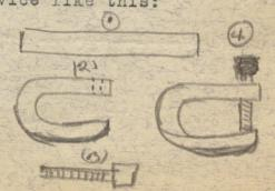
hot on the furnace and bendmit on the anvil with the hammer. It is easy to bend it when it i is red hot. When you make the screw you have to make it out of a square piece of iron so you have to put it on the lathe and make it round. After you make it round you put on the thread. I skip a grade and I have do not have Spanish no more-until the mith ninth grade.
