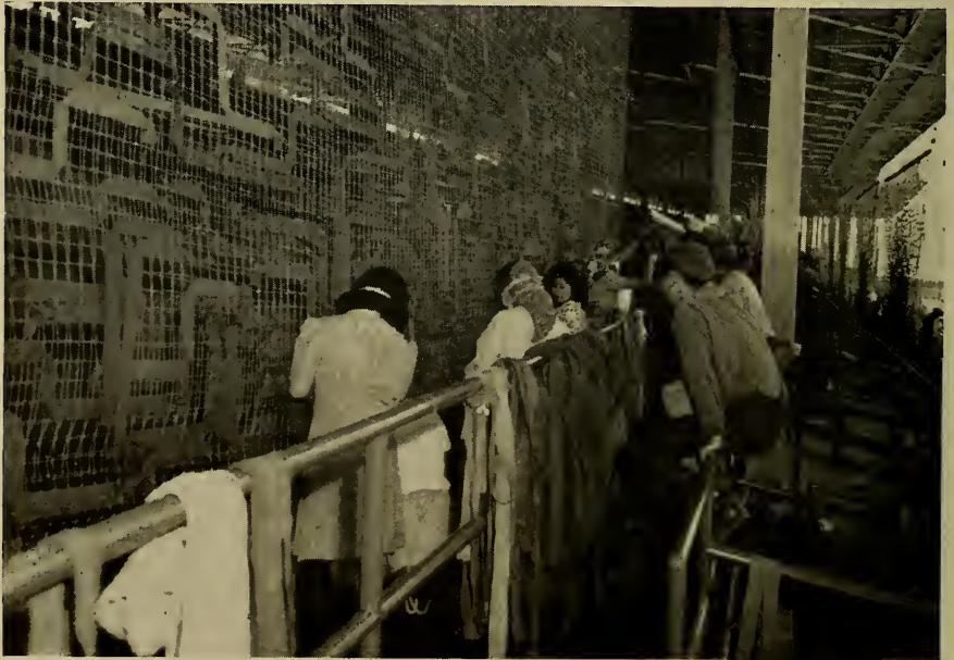
FIGURE 132: Making camouflage nets at Santa Anita (California) Assembly Center. This work is termed "garnishing." A "pattern net" with a design woven into it is first set up and over it a plain net is placed. Weavers worked burlap strips into the top net, following exactly the pattern net as to color and weaving design. The women at work are American-born Japanese.
