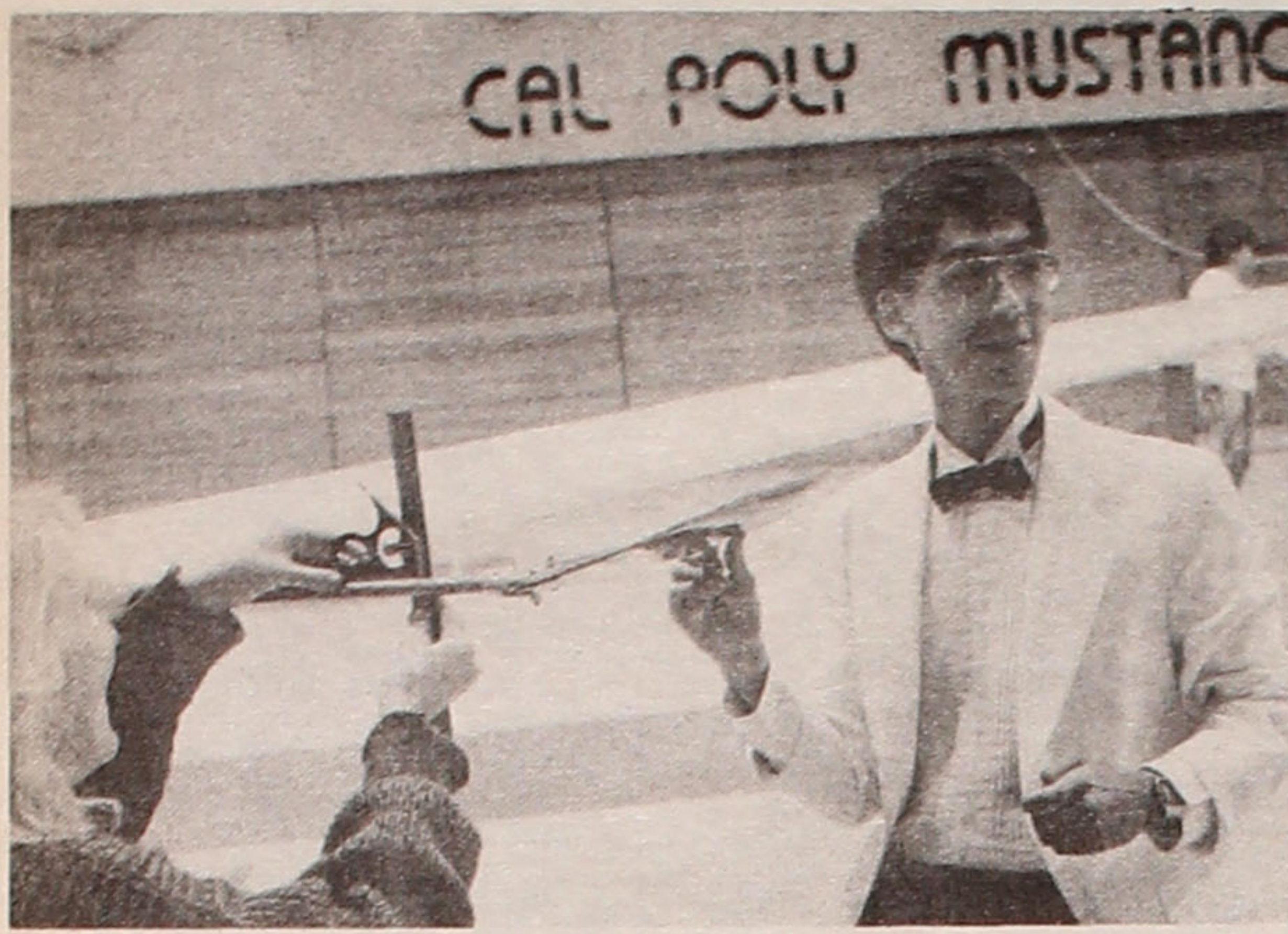
FIRST HUMAN-POWERED HELICOPTER FLIGHT —at Cal Polytech/San Luis Obispo, Calif., on 11/12/89: Designer of the DaVinci III and Project Manager, Neal Saiki, with an assistant, as they work on attaching the propellers to the end of the helicopter rotor.
